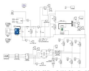
Figure 11: Simulink Model of Micro Grid in Islanding Mode
