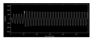
Figure 12: AC Side Voltage of the Main Converter with Constant Solar Irradiation Level and Variable DC Load
