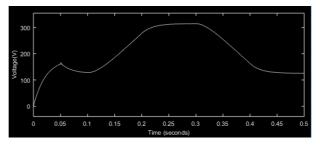
Figure 8: Output Voltage of Boost Converter
