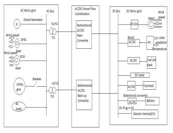
Figure 1: The AC/DC Micro Grid System
